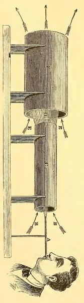
current. D, Second primary current of air passing from C into F. E, E, Induced currents, resulting from the primary current the larger tube C. B, B, Arrows indicating the direction of the induced currents of air, which are put in motion by the primary D. From F the air escapes into open space, as indicated by the arrows Explanation.—A, Small tube through which air is blown, constituting a primary current, represented as passing into
